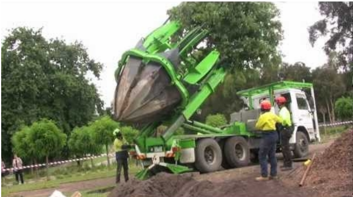
Figure 27: Example of transplanting established trees from one site to another using a tree spade (ArborCoAustralia, 2012)
